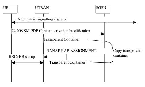
For the transfer of these parameters between source RNC/ BSS and target BSS / RNC at Hand-Over / SRNS relocation, a possible solution could be that independently from the current Radio Access Technology (GERAN / UTRAN) used at PDP context activation, the UE sends the media parameters for RAN both for GERAN and UTRAN technologies allowing further Hand-Over / SRNS relocation / directed retry without any further exchange of these parameters between the UE and the network.
